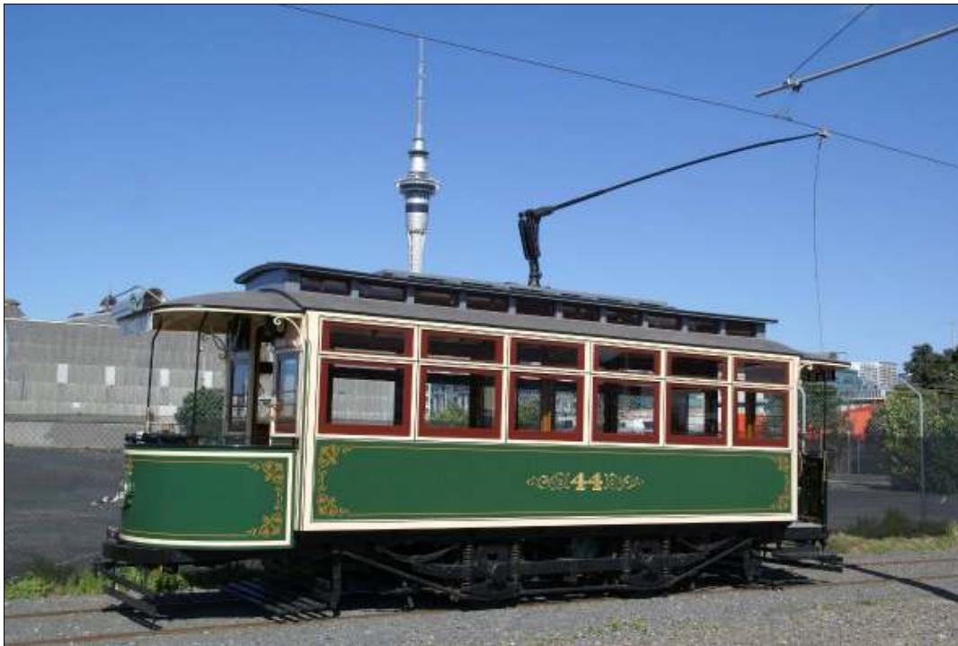
Auckland Tram number 44, built in Ponsonby in 1906 by the Auckland Tramways. This was the first tram to be built in Auckland. Restored by the Western Springs Tramway, MOTAT.
